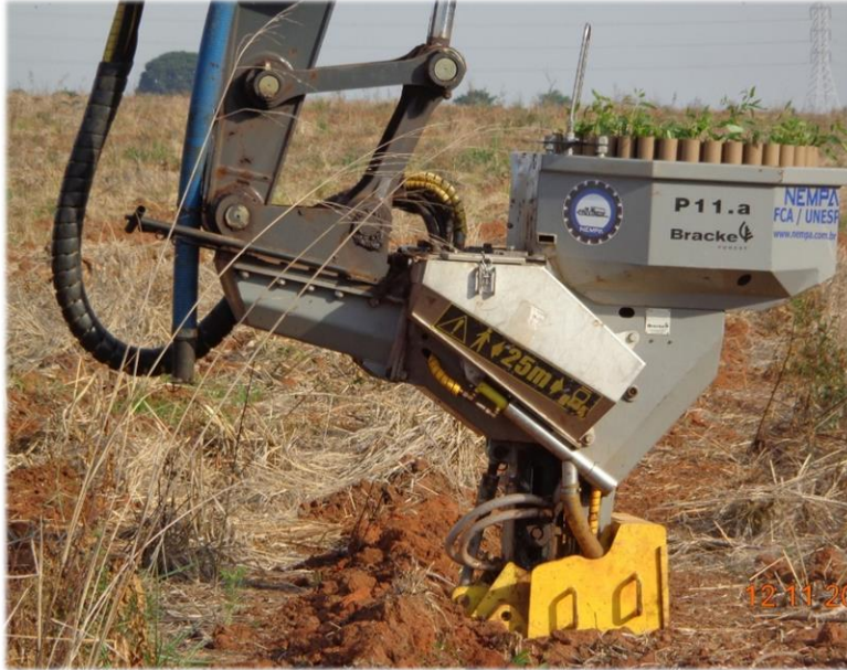
Bracke planter for regeneration work in Brazil
