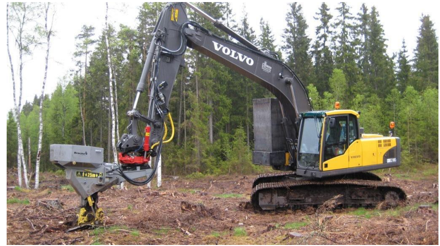
Bracke Planter on tracked excavators
