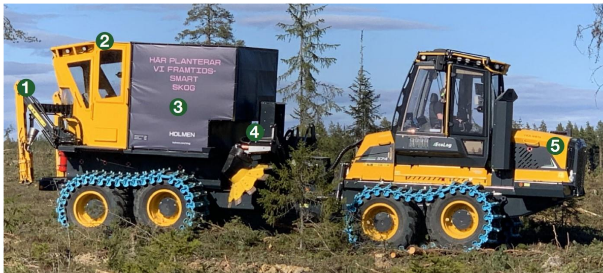
1. Two planting arms | 2. Seedling feeding operator | 3. Seedling storage | 4. Midiflex scarifier | 5. Base machine
